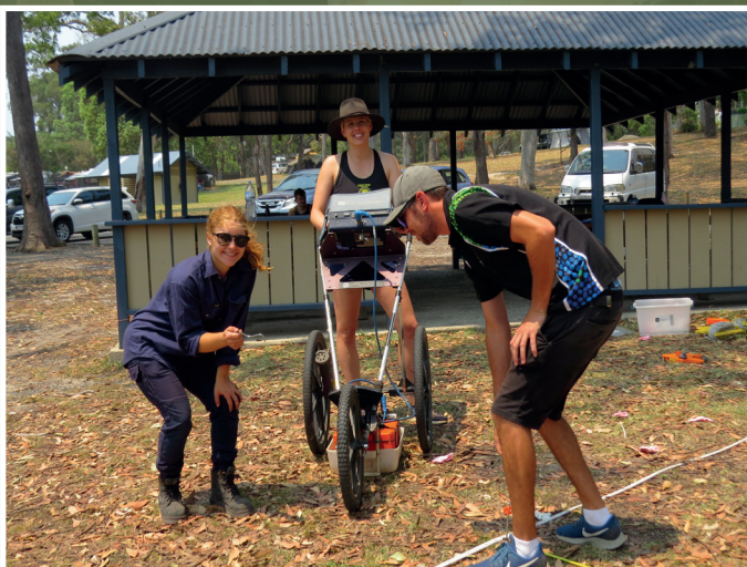
The Coffs Harbour and District Local Aboriginal Land Council Green Team with Elle Lillis undertaking GPR survey at Moonee Beach
