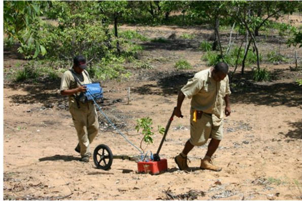
Fig. 7 Data collection using the 400 MHz antennas with a survey wheel attached, connected to the SIR-3000 system control unit with a blue cable
